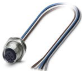
Sensor/actuator flush-type socket, 5-pos., M12 SPEEDCON, A-coded, rear/screw mounting with M16 thread, with 0.75 m TPE litz wire, 5 x 0.34 mm 2
