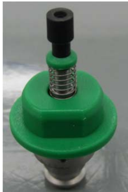
Figure 7. Pick and place machine settings for Juki KE2080L in combination with the off-the-shelf nozzle 505 (inner diameter: 1.7mm, outer diameter: 3.5mm).
