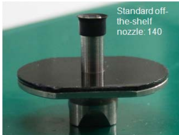
Figure 6. Pick and place machine settings for Panasonic CM402 in combination with the off-the-shelve nozzle 140.
