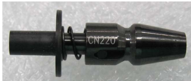
Figure 4. Pick and place machine settings for Samsung SM421 in combination with the off-the-shelf nozzle CN220 (inner diameter: 2.2mm, outer diameter: 3.6mm).
