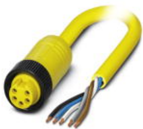
Power cable, 5-position, PVC, yellow, free cable end, on Socket straight 7/8"-16UNF, cable length: 5 m
