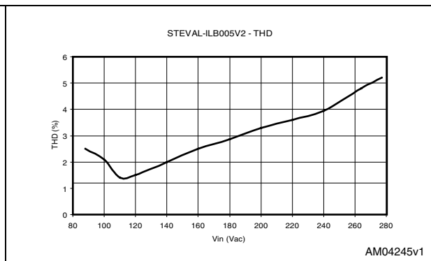
Figure 17. Input performance - total harmonic distortion
