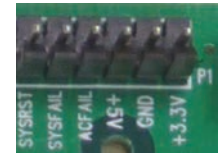
6-Pin Utility Connector On rear of Backplanes
