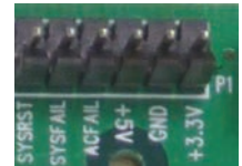
6-Pin Utility Connector On rear of Backplanes
