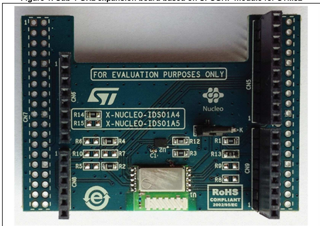
Figure 1. Sub-1 GHz expansion board based on SPSGRF module for STM32
