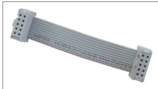
Figure 3: Flat cable with IDC10 connectors
