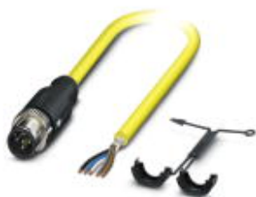
Sensor/Actuator cable, 5-position, PVC, yellow, shielded, Plug straight M12 SPEEDCON, A-coded, on free cable end, Cable length: 10 m
