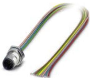
Sensor/actuator flush-type plug, 8-pos., M12 SPEEDCON, rear/screw mounting with M12 thread, with 0.5 m TPE litz wire, 8 x 0.25 mm 2
