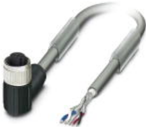
Bus system cable, CANopen®, 5-position, PUR halogen-free, Gray RAL 7001, shielded, Free cable end, on Socket angled M12-SPEEDCON, A-coded, Cable length: 2 m
