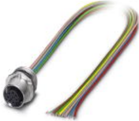
Sensor/Actuator flush-type socket, 8-pos., M12-SPEEDCON, A-coded, front/screw mounting with M16 thread, with 0.5 m TPE litz wire, 8 x 0.25 mm 2
