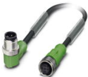
Sensor/actuator cable, 3-position, Variable cable type, Plug angled M12, A-coded, on Socket straight M12, A-coded, PIN 2+4 bridged, cable length: Free input (0.2 ... 40.0 m)
