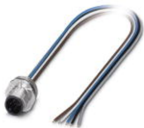
Sensor/actuator flush-type plug, 5-pos., M12-SPEEDCON, A-coded, front/screw mounting with M16 thread, with 0.5 m TPE litz wire, 5 x 0.34 mm 2
