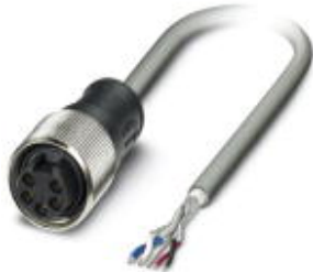
Bus system cable, DeviceNet, 5-position, PUR halogen-free, Gray RAL 7001, Free cable end, on Socket straight 7/8"-16UNF, Cable length: 15 m
