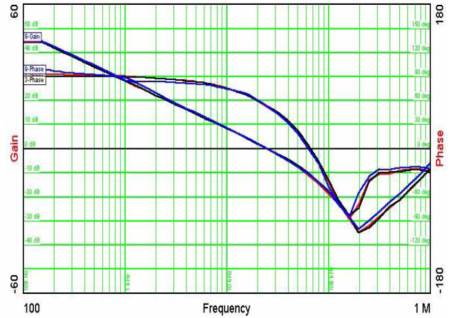
FIGURE 79. OPEN LOOP RESPONSE FOR 2.64V @6A CONSTANT CURRENT LOAD. RED-48V, BLUE-75V, AND BLACK-36V
