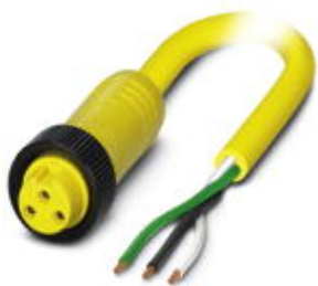
Power cable, 3-position, PVC, yellow, free cable end, A - standard, on Socket straight 7/8"-16UNF, cable length: 1 m
