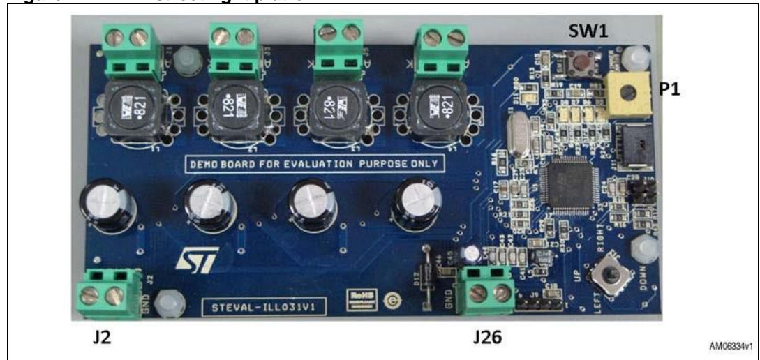
Figure 12. LED street light platform
