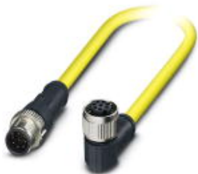
Sensor/Actuator cable, 8-position, PVC, yellow, Plug straight M12 SPEEDCON, A-coded, on Socket angled M12 SPEEDCON, A-coded, Cable length: 1.5 m
