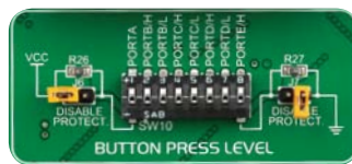
Figure 6-5: Button press level DIP switch (tri-state)
