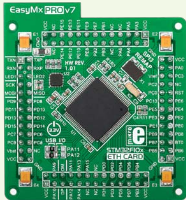
Default 100-pin ETH MCU card with STM32F107VCT6
