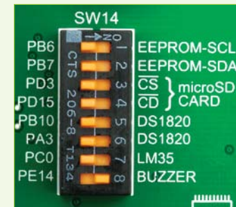
Figure 25-2: push SW14.8 to ON position to connect Piezo buzzer to PE14
