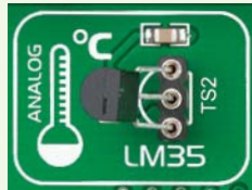
Figure 21-2: LM35 correctly placed in socket
