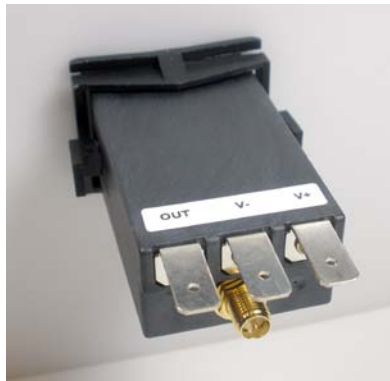
Figure 26. WPMM Panel Mount – Back View In Place
