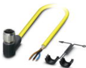
Sensor/Actuator cable, 3-position, PVC, shielded, free cable end, on Socket angled M12 SPEEDCON, A-coded, Cable length: 5 m
