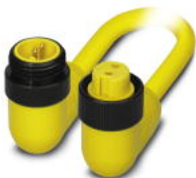
Power cable, 2-position, PVC, yellow, Plug angled 7/8"-16UNF, A - standard, on Socket angled 7/8"-16UNF, cable length: 5 m
