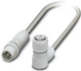
Sensor/Actuator cable, 4-position, PP-EPDM halogen-free, Gray RAL 7035, Plug straight M12, A-coded, on Socket angled M12, A-coded, with 3 LEDs, Cable length: 0.6 m, Hygienic design, with plastic knurl
