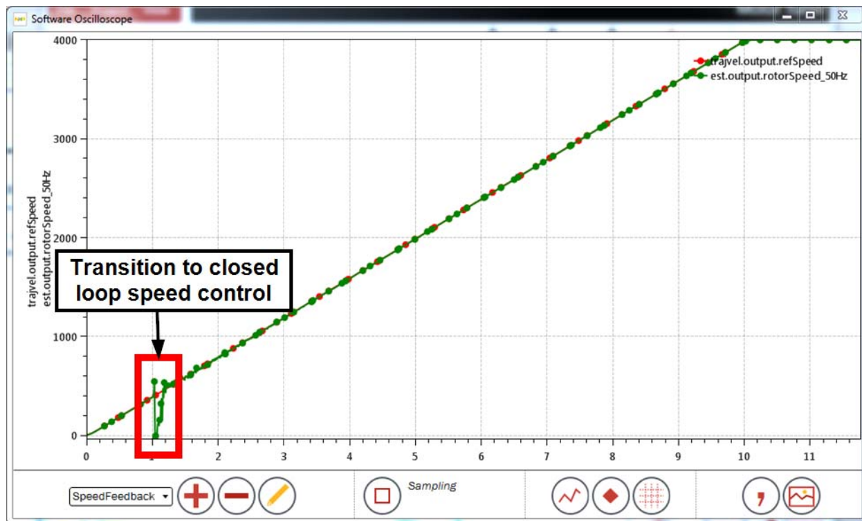
Figure 81. Transition from open to closed loop control
