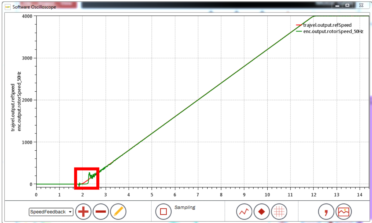
Figure 82. Sensored velocity operation during Spin!
