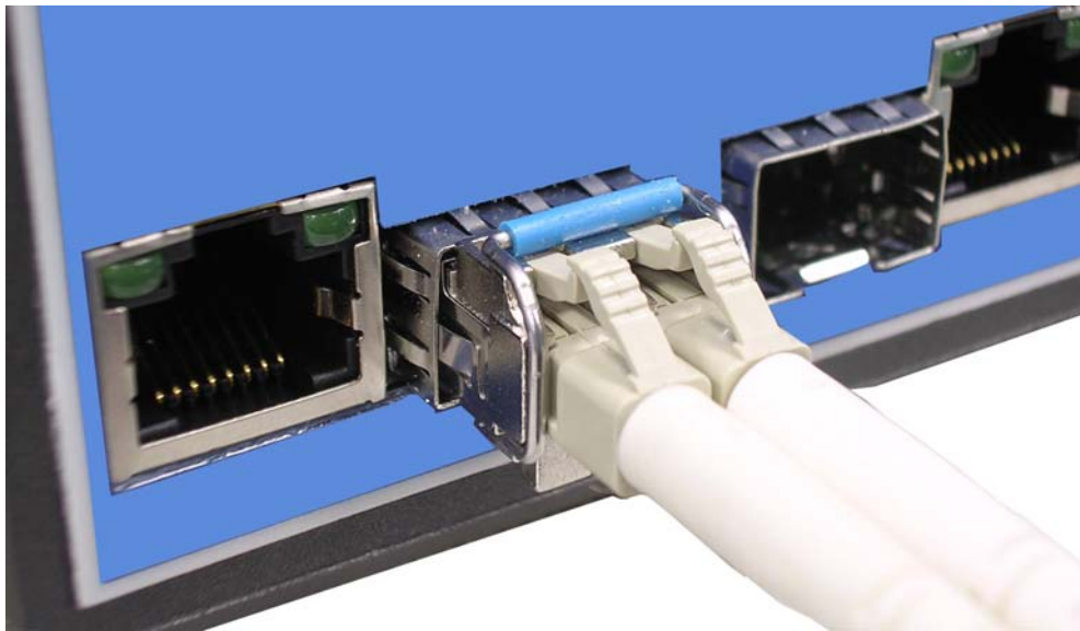
Figure 2.10: LC connector to the transceiver
