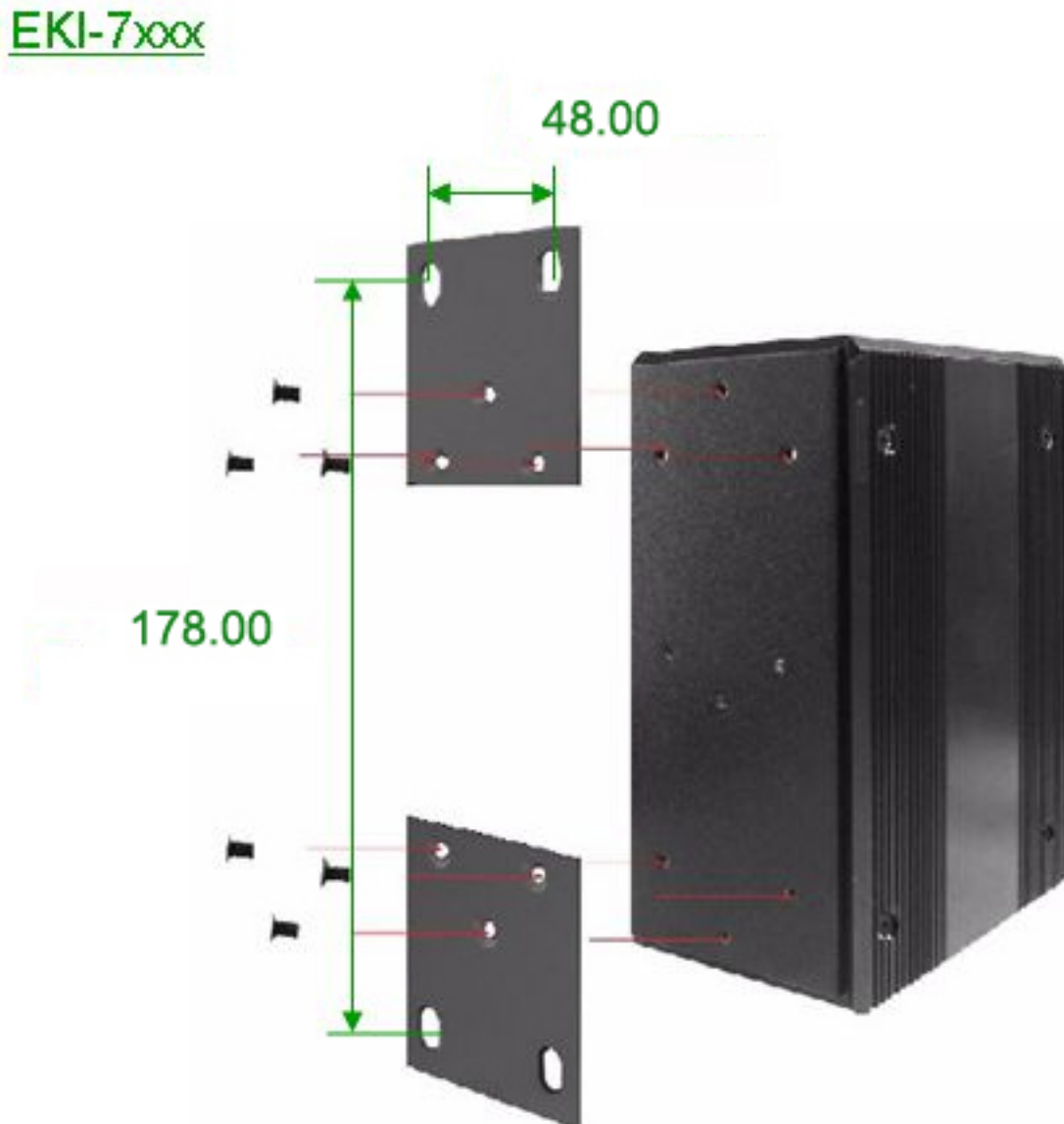
Figure 2.5: Combine the Metal Mounting Kit
