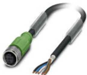
Sensor/actuator cable, 5-position, PUR halogen-free, black-gray RAL 7021, shielded, free cable end, on Socket straight M12, A-coded, cable length: 30 m
