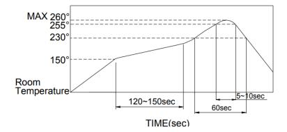
■ The temperatures defined above are the temperatures measured on the surface of the Printed Circuit Board. There are cases where the printed circuit board's temperature differs greatly from the temperature of the switch. Critical note: the switch's surface temperature must not exceed 260°C.
