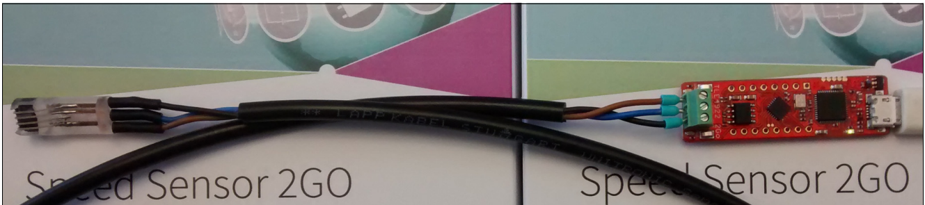
Figure 26 Hardware of “SPEED SENSOR 2 GO”: Module and pcb
